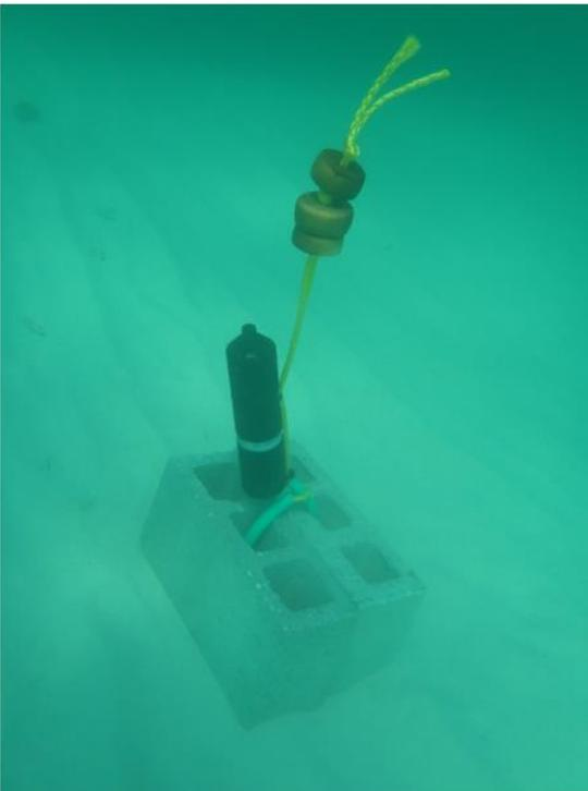
**An acoustic receiver is anchored to the ocean floor and held upright with a couple floats.**
